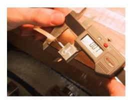
The gouging machine will have finished its work when there is no cane being cut in BOTH DIRECTIONS. At this point, inspect the thickness in the CENTER with a micrometer. The gouge CENTER THICKNESS should be 0.60mm. This can vary slightly to taste. I also check this side thickness of the cane after shaping it. This measurements should be around 0.50mm.
