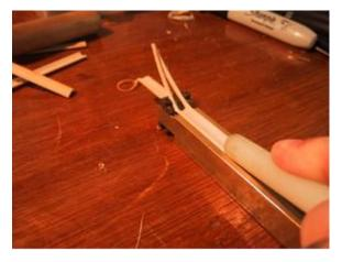
The piece of cane should be 8.0mm across the flat surface. This is VERY IMPORTANT. If the cane is too wide, the machine will not gouge in an optimal fashion. See PLANING YOUR CANE in the Gouger University's Freshman Class #1 for more information on this.
