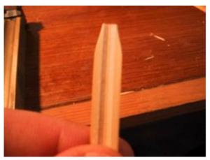
Once you cane is planed to the appropriate width, you should narrow the ends of the cane before gouging. The intent is to allow the blade edge to FEED into the side part of the gouge curve. I cut off the outer third on each side starting about one-half inch from the end.
