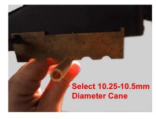
the top surface of the cane. This way I can use the light to illuminate the cane so that inspection of the diameter is easier. Measure down the whole length of the tube to make sure the diameter is consistent.
