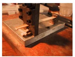
Another reason for chopping the cane at both ends is the section of the cane that you want to use may be located somewhere in the middle of the piece of cane that you cut from the tube. The cane is generally cut in the cane fields near the knots on the stalk. Since the grain is merging into the knots, the cane will sometimes have a curve in it near these locations.
