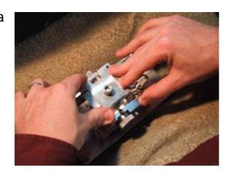
The Opus1 Gouger is a DOUBLE RADIUS gouger. It is designed to have the cane flipped every 5 or so passes of the carriage. This is done to help insure symmetry in the gouge. Both walls of the cane's finished gouge curve are cut with the same half of the blade curve.
