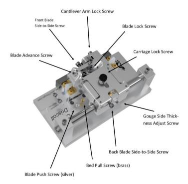
handles a specific adjustment to manipulate the measurements of the gouge curve. There is only one screw used to make any specific measurement change. This allows you to UNDO a specific adjustment that you might make and not find to your satisfaction. On other designs, you will need to move multiple screws to make a single adjustment, which becomes impossible to undo unless you are skilled
